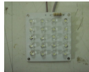
Gambar 14. Lampu LED 0,75 W
