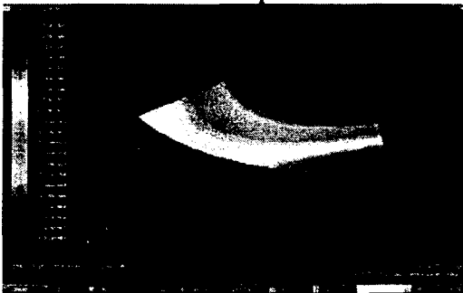
Gambar 1. Distribusi tekanan statis sudu turbin model 1 ( steady )
