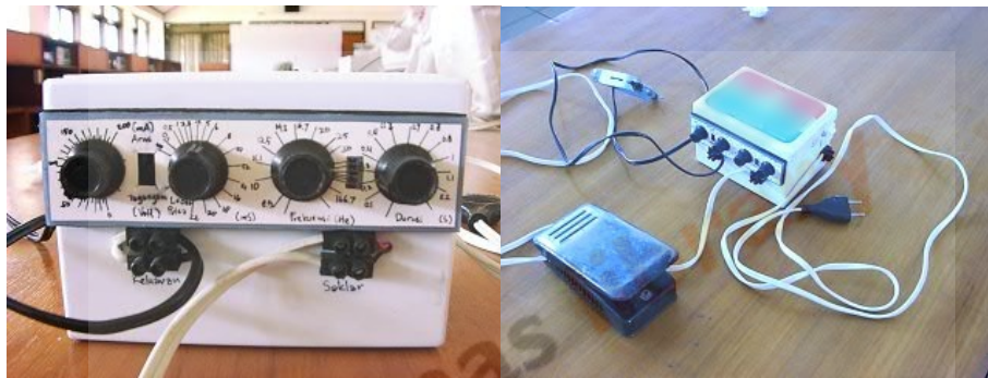
Figure 18 Photograph of the constructed electroconvulsive device.
