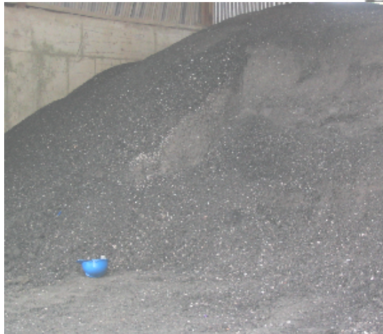
Figure 2 Sampling of stockpiled Reclaimed Asphalt Pavement
