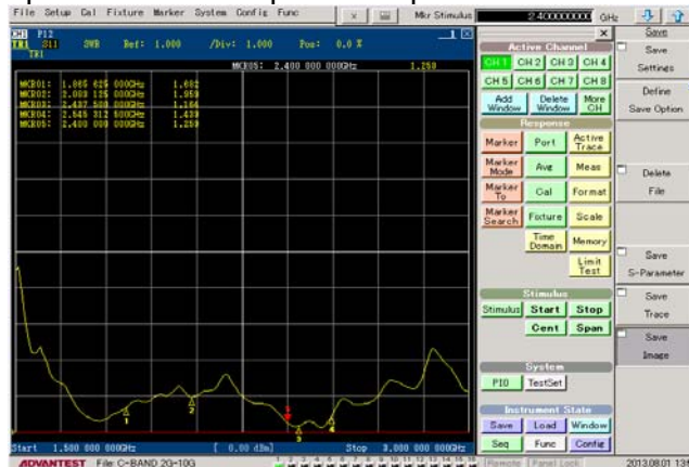
Gambar 8. Hasil Pengukuran Standing Wave Ratio (SWR)
