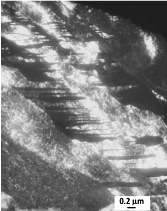
Fig. 10. Bright field TEM image after austenising at 1250 °C and deformation at 1000 °C showing microtwins.
