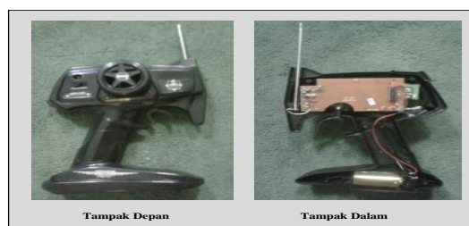
Gambar 3. Sistem Pemancar Radio Remote Tilting Antenna
